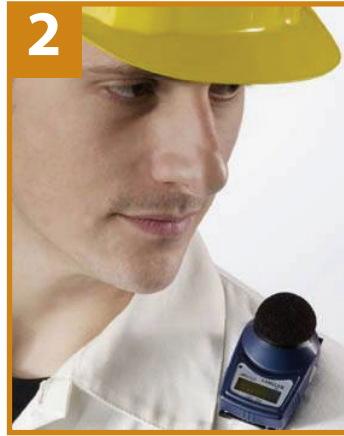
Use a noise dosimeter that is attached to a worker while conducting the test.
