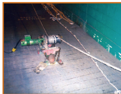
View of tugger with sample of kinked rope on the floor nearby.
